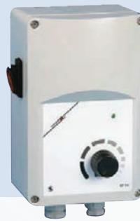
Electronic speed controller for the speed control of single phase motors by varying supplied voltage
